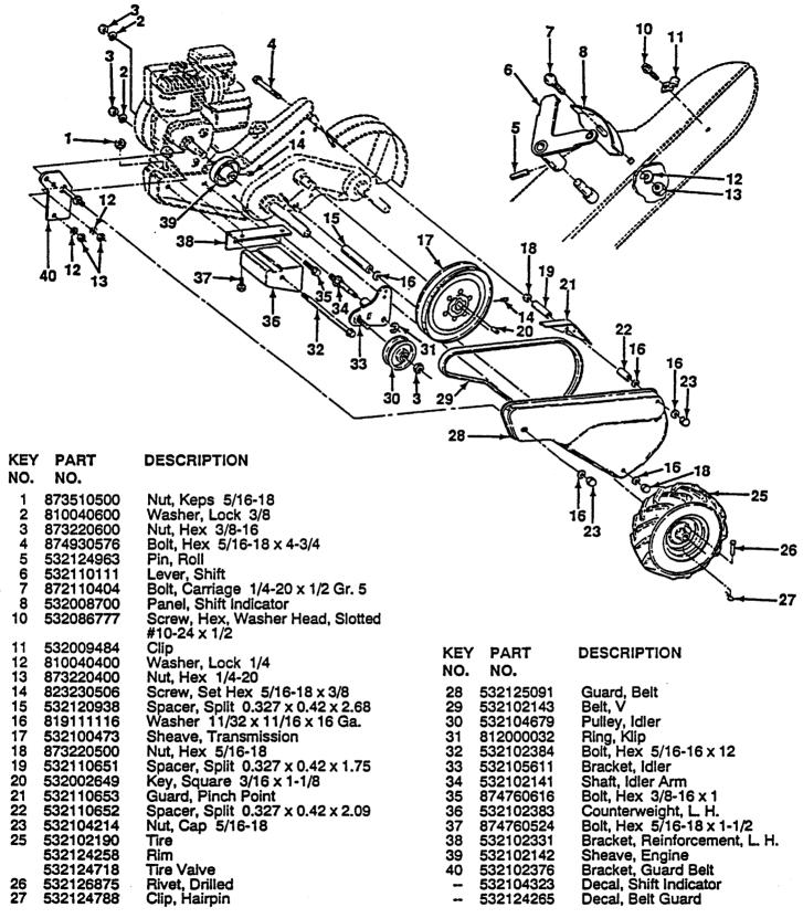
NOTE: All component dimensions given in U.S. inches. 1 inch = 25.4 mm
